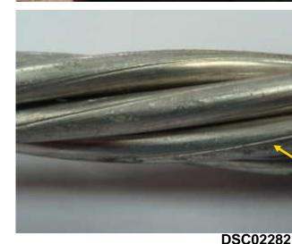
This is aluminium conductor. Below is the unique marking found on Eskom aluminium conductor – to the naked eye it simply looks as if the conductor is scratched.
