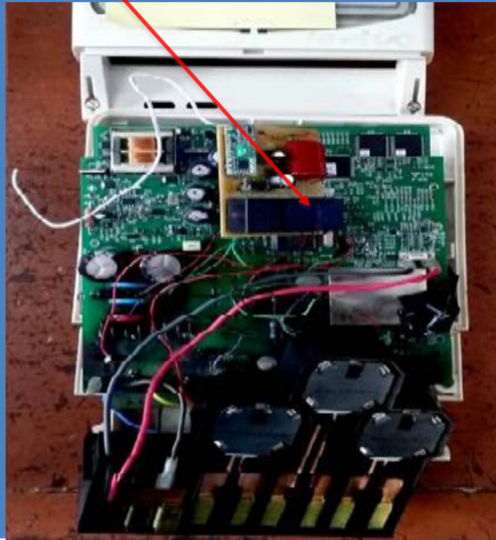
Foreign circuit controlling energy registers to limit energy measurement
