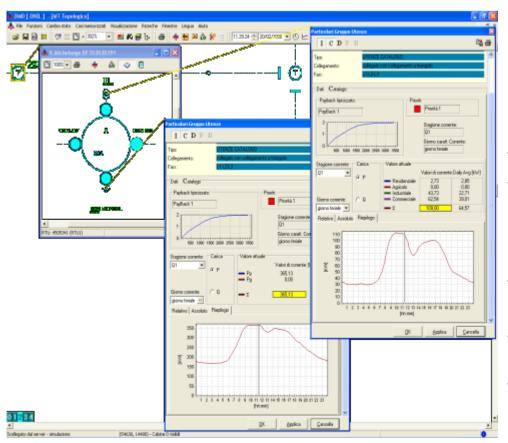
DMS main functionalities are topology analyzer, load flow, state estimation, optimal feeder reconfiguration, voltage control, short circuit calculation.
